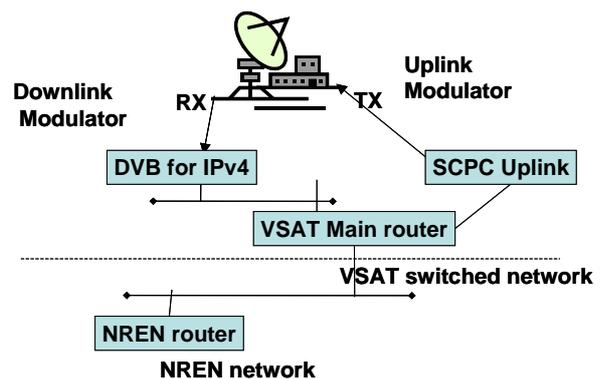
Figure 4. Schematic of Equipment used for IPv4 at the partner sites
