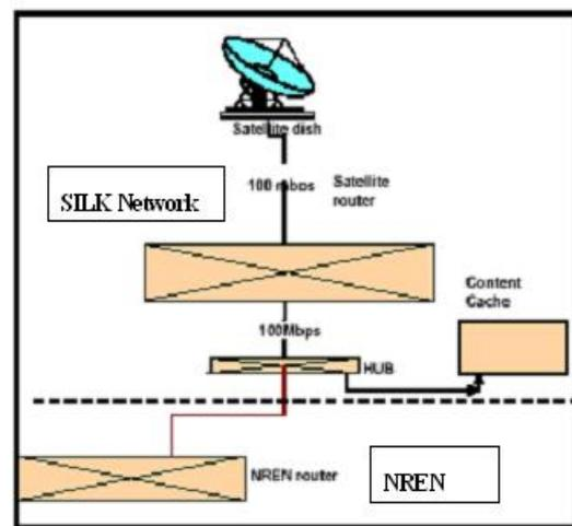
Fig. 2. Schematic of Equipment at each Remote
