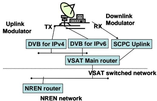
Figure 5. Schematic of Equipment used for IPv4/6 at the hub site
