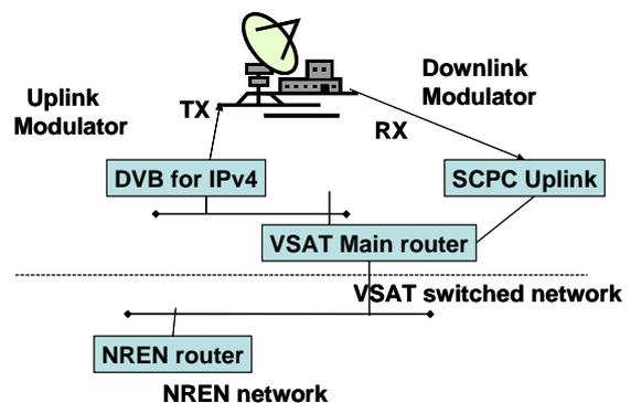
Figure 3. Schematic of Equipment used for IPv4 at the hub site
