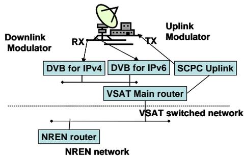
Figure 6. Schematic of Equipment used for IPv4/6 at the partner site sites
